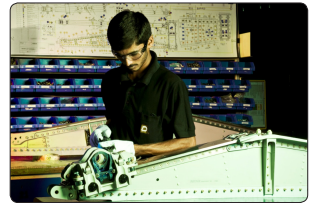
Assembly of Flap-Track-Beams for Airbus A320 Single Aisle Aircraft at Dynamatic, Bangalore, India
