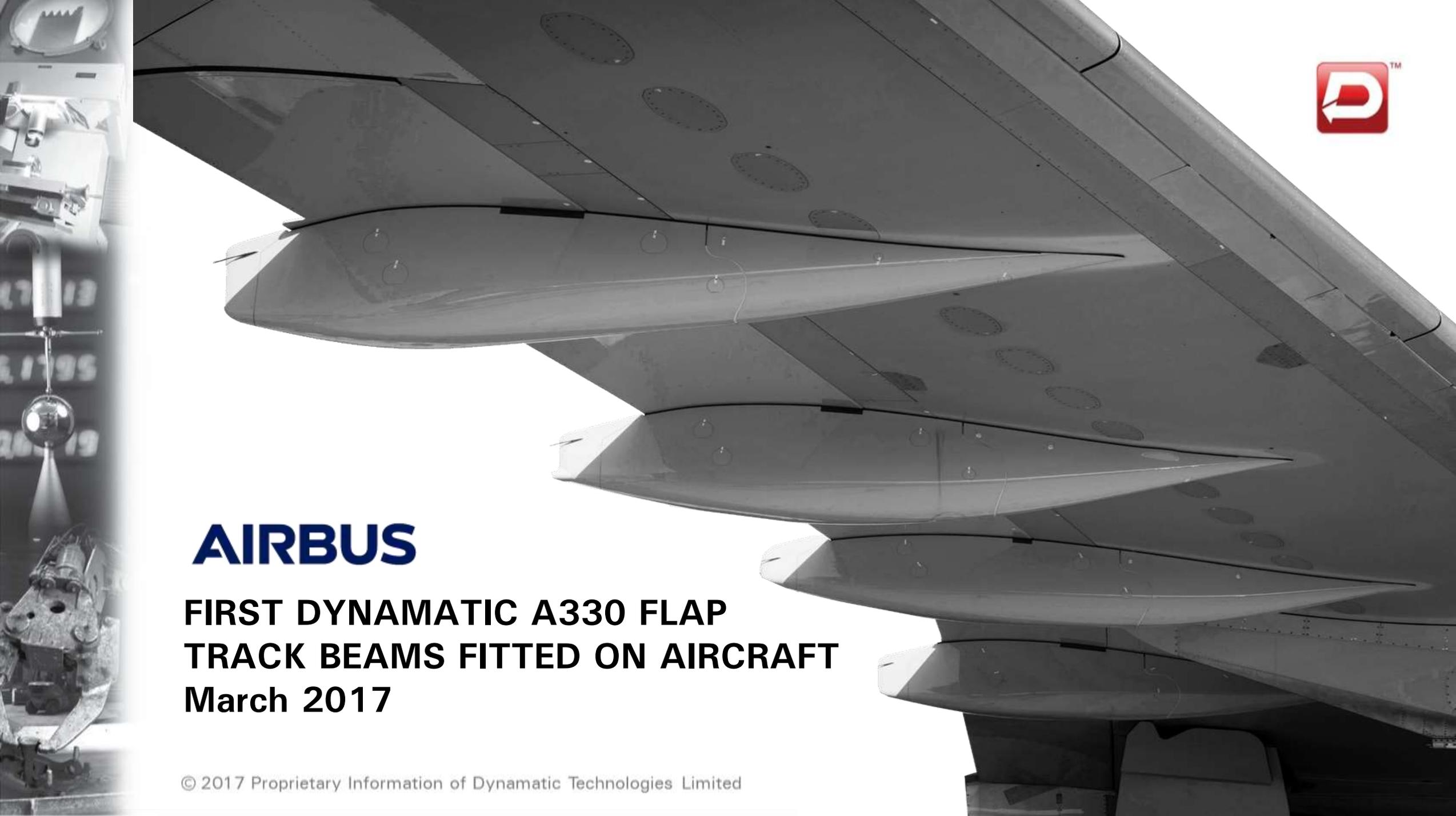
A black and white photograph showing the underside of an aircraft wing with three flap track beams. The beams are curved and mounted to the wing structure. The background is white. On the left side, there is a vertical strip showing a close-up of a flap track beam mechanism and a small globe on a stand.
