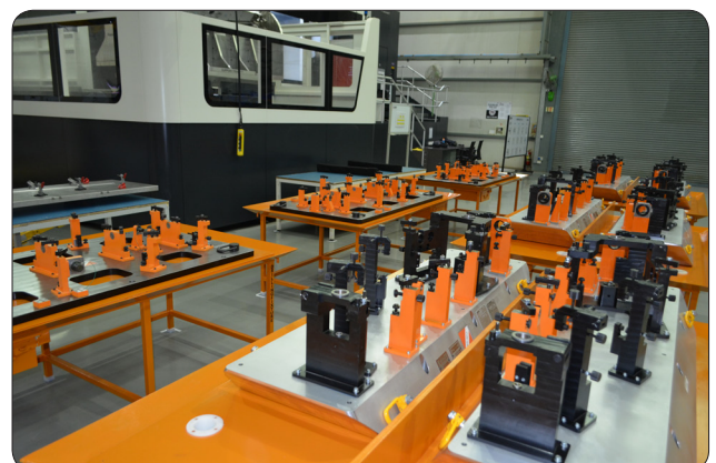
Above & Below: Assembly line established at Bangalore, India, to produce Redesign Flap-Track-Beams for the Airbus A320 family.
