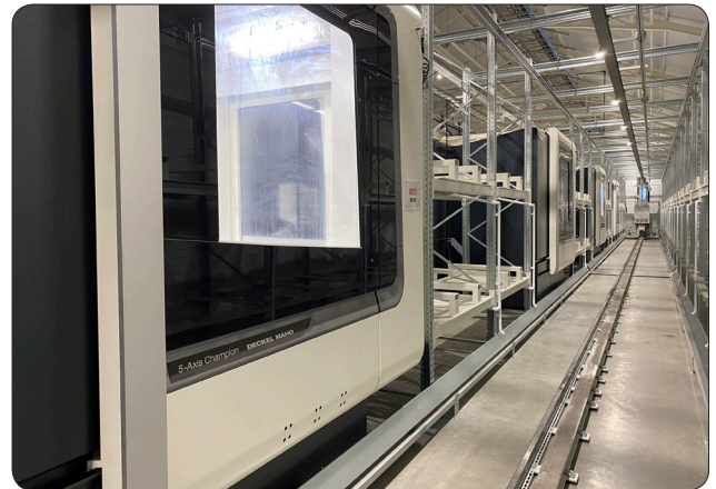
Advanced Robotic machining line at Swindon, UK, to produce Monolithic parts for the Airbus A320 family.
