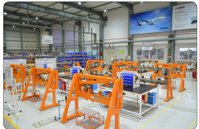
Above & Below: Assembly line established at Bangalore, India, to produce Redesign Flap-Track-Beams for the Airbus A320 family.
