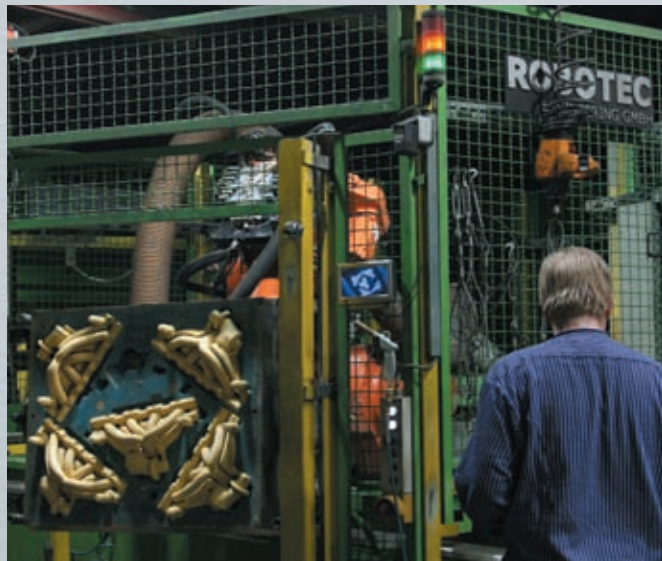
High Precision Robotic Core Setter in the GFD Moulding Line at Eisenwerk Erla GmbH, Germany.
