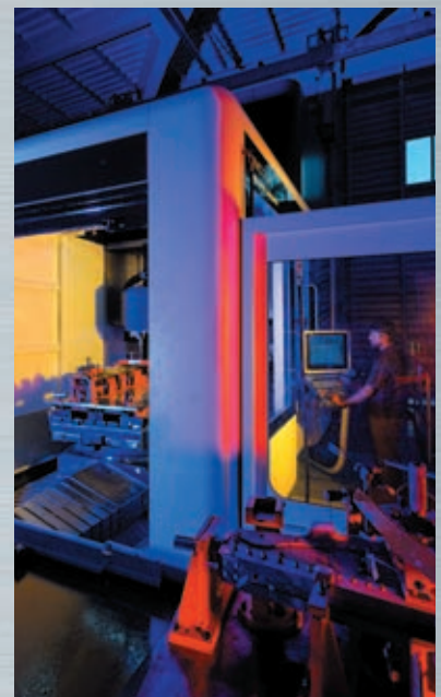
Machining of the Flap Track Beam for the Airbus Single Aisle Aircraft at Dynamatic-Oldland Aerospace™
