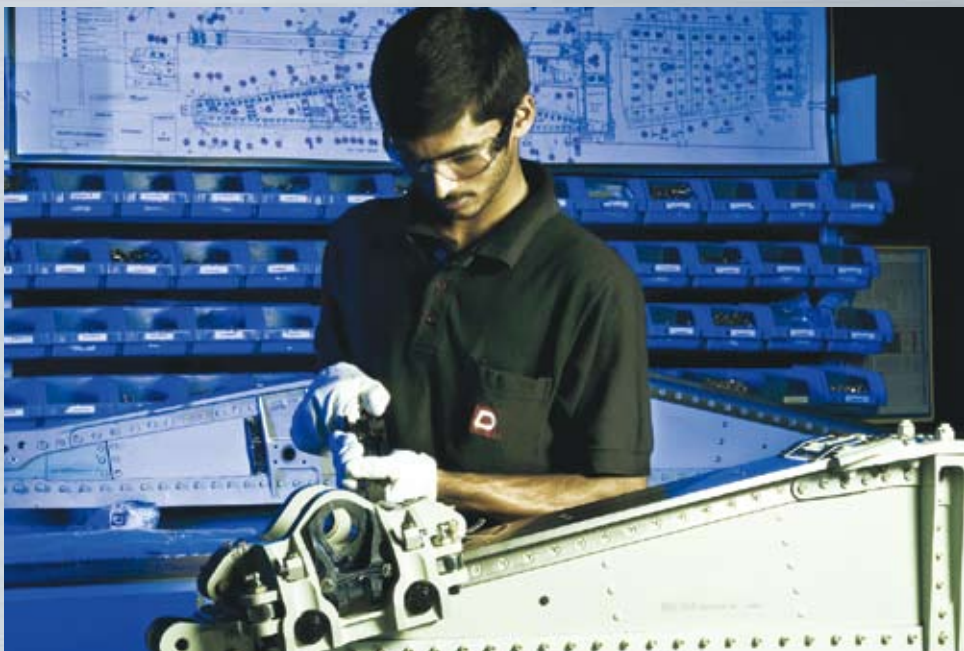
Carriage Assembly on a Flap Track Beam for the Airbus A320 Single Aisle Aircraft at Prana, Dynamatic Aerospace®
