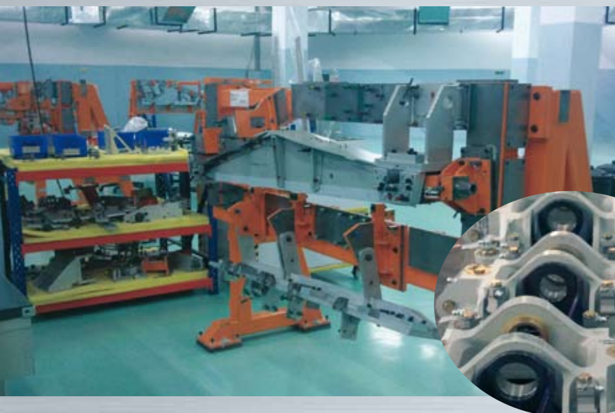
The Airbus A320 Flap-Track Beam under production at 'Prana', Dynamatic's new Aerospace facility
