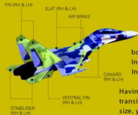
Pictured above is the Sukhoi 30-MKI, fighter-bomber, with the major airframe structures manufactured by Dynamatic Aerospace® shown shaded.
