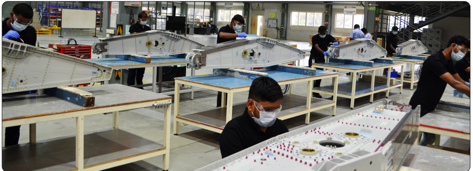
Airbus A330 Flap Track Beam Assembly Line at Dynamatic Aerotropolis
